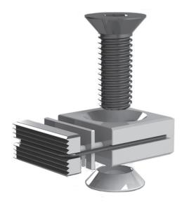
The base M-series clamp is the same size as a standard Tiny Vise<sup>®</sup>, with the same reversible jaw faces (one serrated and one smooth). The 1/4"-thick serrated modular jaw mounts into the smooth face, and each spacer can be inserted to provide adjustment. The modular jaw assembly is held together securely by a tough, durable O-ring, recessed in a protective groove. The modular jaw can be easily extended to insert or remove the slotted spacers.
