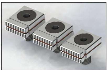
M-series clamps have a 1/4"-thick modular jaw that can be easily extended to insert or remove spacers. Up to three 1/16" spacers can be inserted to provide adjustment.
