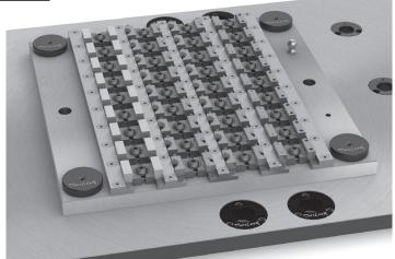
Just like our original Tiny Vise\*, these mini edge clamps grip the side of a workpiece to keep the top clear for machining. Patented design features a slotted countersink to provide strong, reliable clamping force with the easy turn of a hex wrench.
